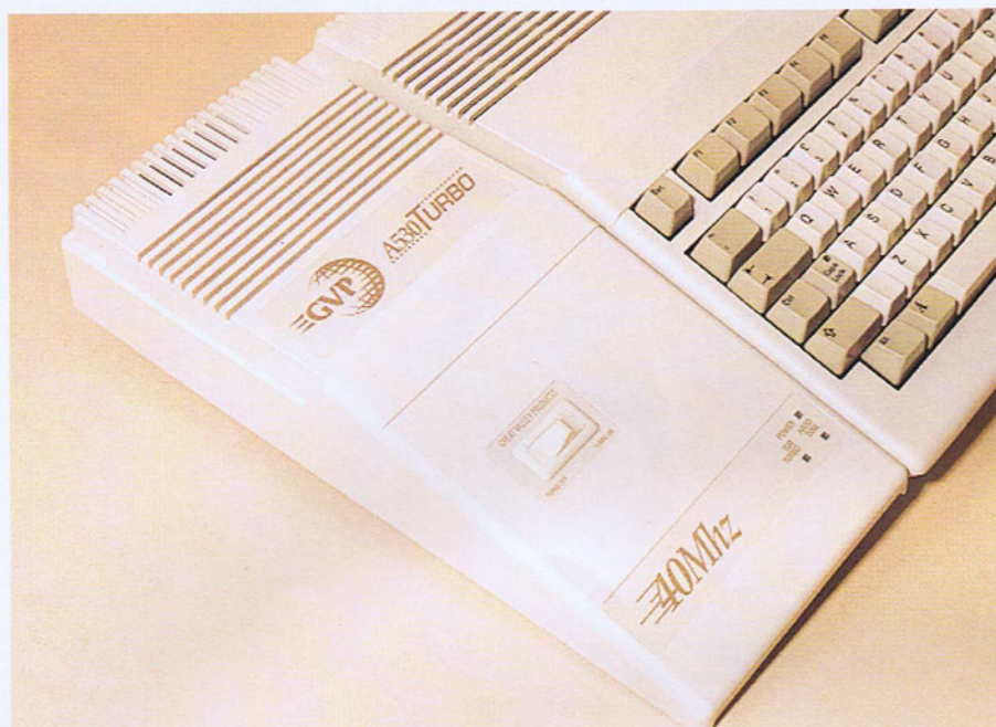
The GVP A530 accelerator can seriously speed up your Amiga as well as providing up to 8Mb of RAM and a hard disk drive of up to 120Mb.
